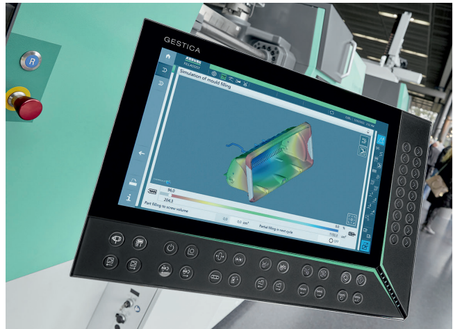
The new tool works on any Arburg injection molding machine with Gestic control. © Arburg
